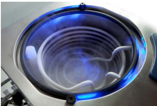
Defrosting a condenser (cold trap) .
